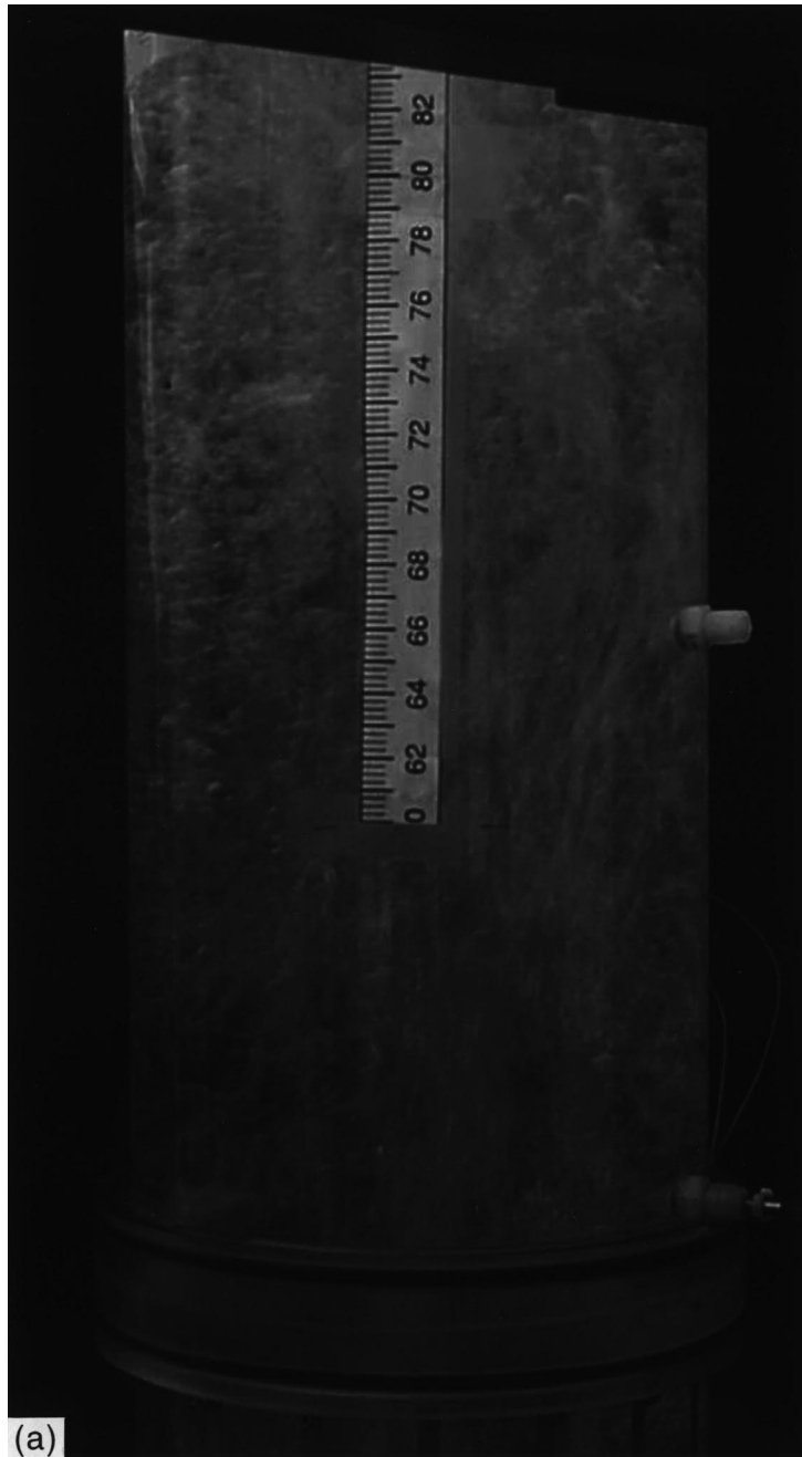
Fig. 13. Churn-turbulent flow conditions in the transparent bubble column at minimum and maximum volumetric flow rates: (a) Q = 420 \text{ cm}^3/\text{s} , (b) 2500 \text{ cm}^3/\text{s} . The vertical scale is in centimeters.
